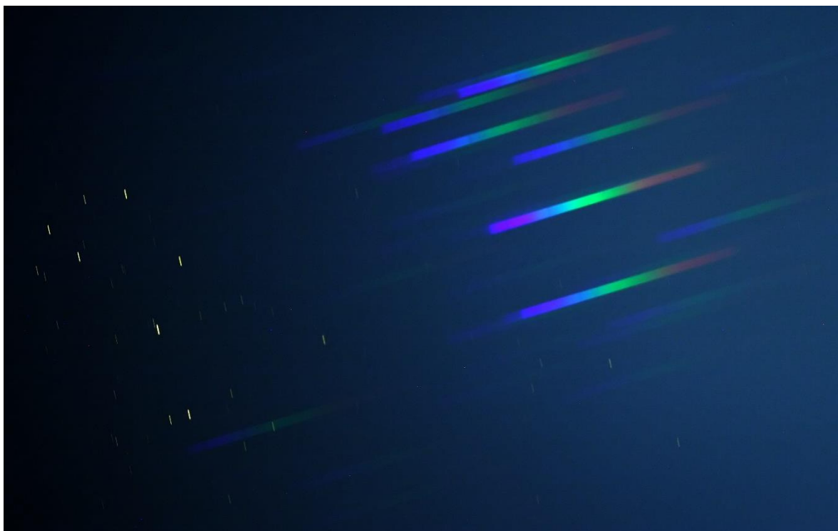
Pleiades (left in image) and associated spectra. Refractor 60/360 with blazed grating and Canon 1000Da, exposed for 30 s at ISO 1600.
